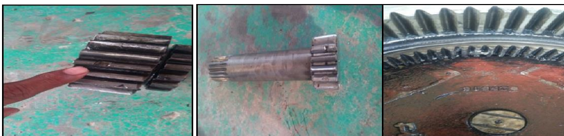
Fig 15. sun gear, shaft gear and ring gear are broken
