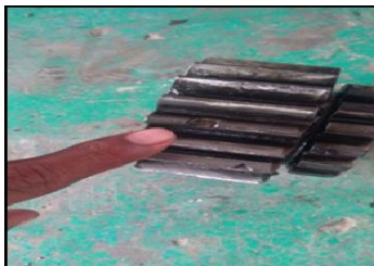
Fig 12. damaged sun gear component
