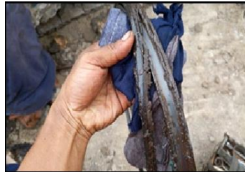
Fig 9. floating seal is damaged
