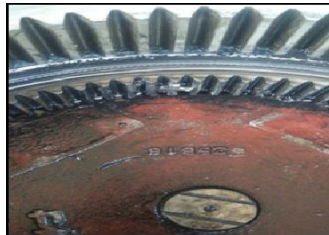
Fig 10. broken ring gear components
