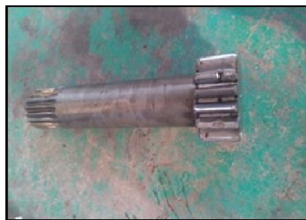
Fig 11. broken shaft gear components
