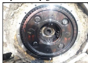
Fig 7. Lube oil burns on planetary gear
