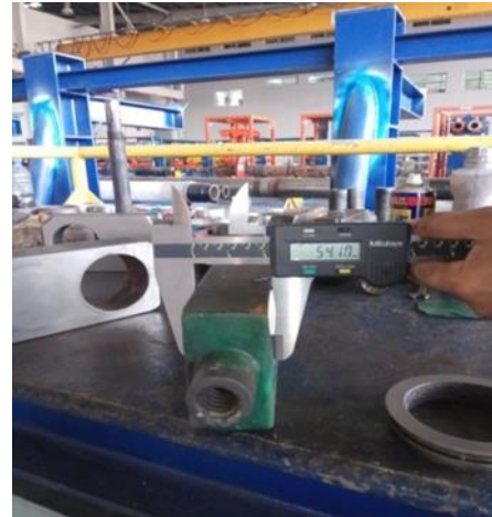
Gambar 8 Ketebalan Standart (Baru) Gate Valve
