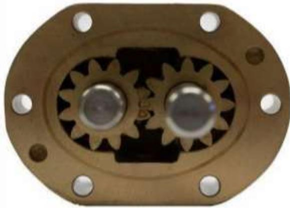
Gambar 3. Pompa gear
