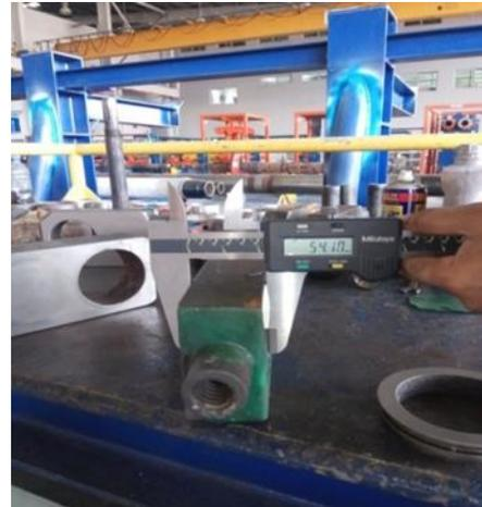
Gambar 8 Ketebalan Standart (Baru) Gate Valve
