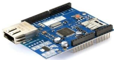
Gambar 3. Arduino Ethernet Shield Board
