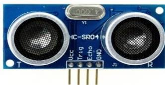
Gambar 4. Sensor SR-04 Ultrasonik
