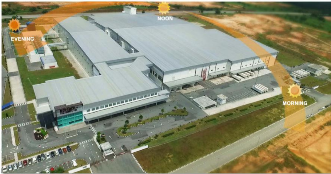
Figure 2. Ariel View of the first GBI Gold Rated confectionery manufacturing facilities in Malaysia (angular view) with indication of sun-path
