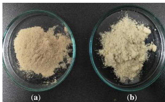
Figure 1. Photograph of (a) raw OPEFB fibres and (b) treated OPEFB fibres.
