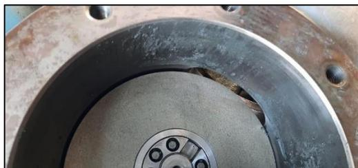
**Gambar 7. Dinding Cylinder Kompresor Kwangshin C-100 mengalami Keausan**
