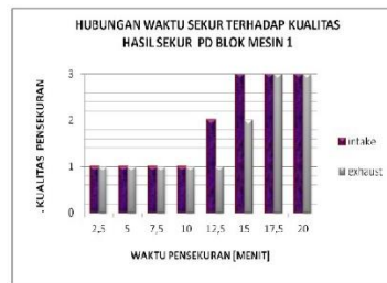
Figure 3. The relationship between staking time and the quality of block 1's staking results
