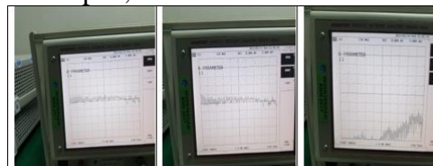
Gambar IV.9. Kalibrasi Internal Network Analyzer (Open, Short, Load)
