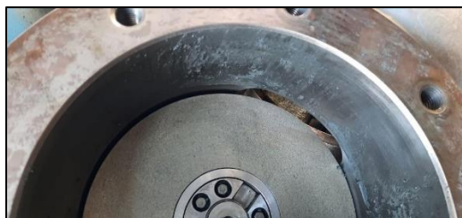
Gambar 7. Dinding Cylinder Kompresor Kwangshin C-100 mengalami Keausan
