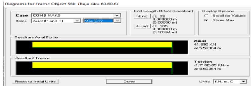
400 401 Figure 25 Axial force. Double elbow steel profile 60.60.6 L 5.44256 kN tension
