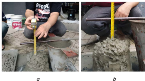
Fig. 1. Slump test: a – for portland cement; b – for portland pozzolan
