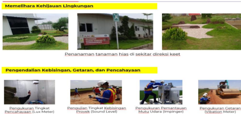
Figure 2. Control of gas emissions, noise, vibration, air and lighting
