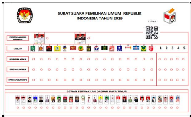
Figure 6: New ballot paper layout design 0.12474-meter square, the function just like a computer answer sheet. It is a combined 5 type ballot used before. And equipped with QR Code feature to avoid a forgery (double print or double recording)
