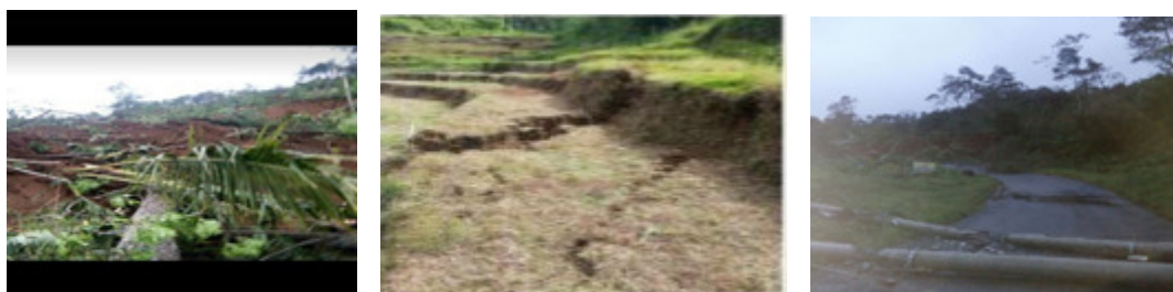
Figure 1 2 3 Type of soil cracks during dry season, expands and landslides during rain
