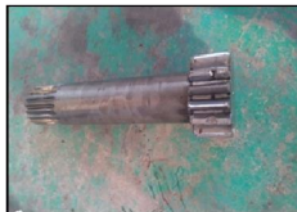
Fig 11. broken shaft gear components
