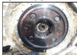
Fig 7. Lube oil burns on planetary gear
