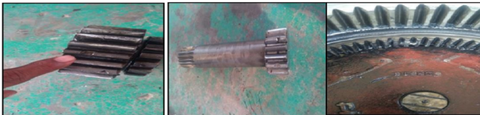
Fig 15. sun gear, shaft gear and ring gear are broken
