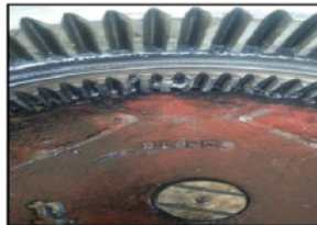
Fig 10. broken ring gear components
