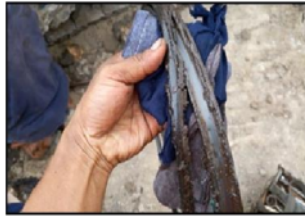
Fig 9. floating seal is damaged
