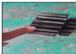
Fig 12. damaged sun gear component
