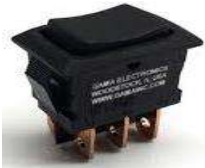
Gambar II.21 Gambar Switch On-Off-On
