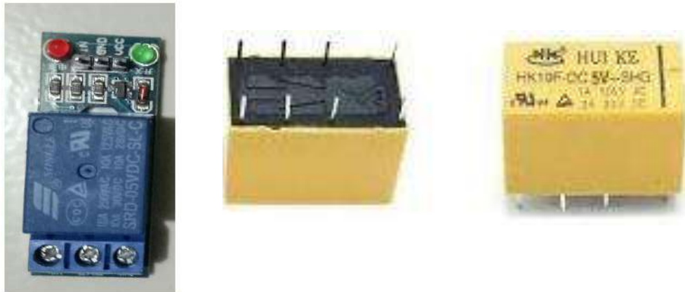
Gambar III.16 Gambar Driver Relay 5 volt
