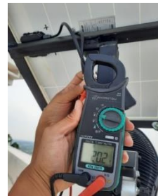
Gambar 3. 19 Pengujian Panel Solar Cell
