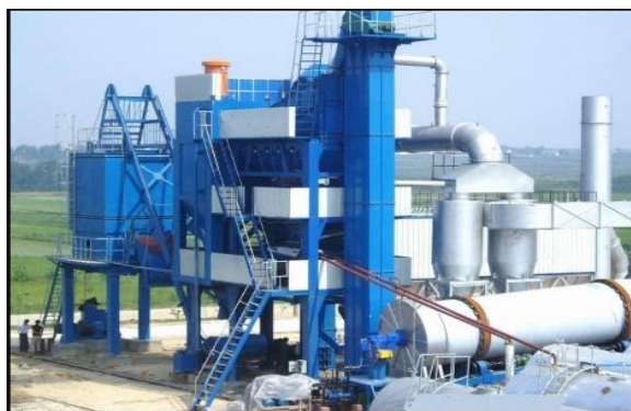
Gambar 4.29 Asphalt Batching Plant
