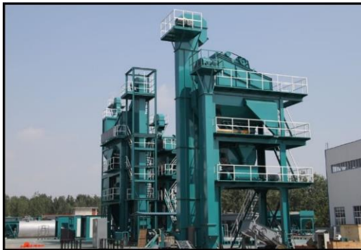
Gambar 4.31 Continuous Asphalt Mixing Plant
