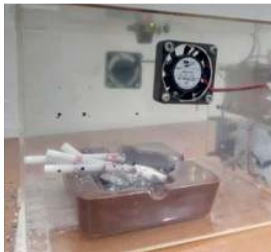
Figure 6. Indoor CO 2 Gas Control System Test
