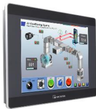
Gambar 3 Human Machine Interface [3]
