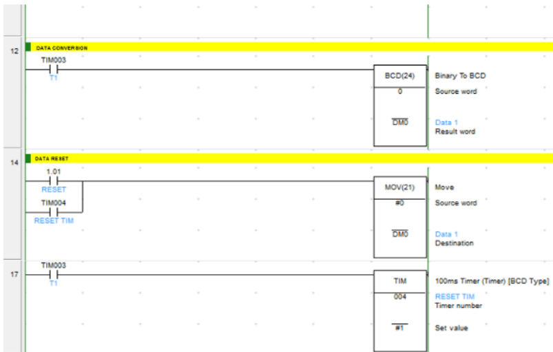
Figure 7. Ladder Diagram 2 of Detector Input
